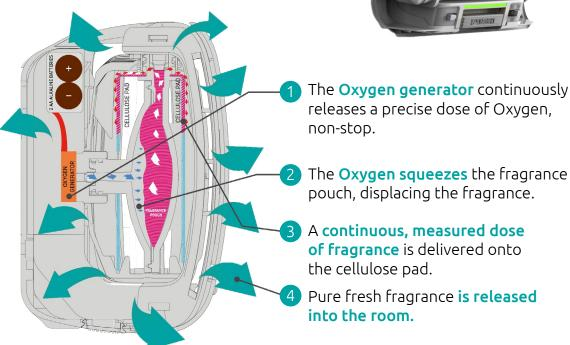
Unlike other traditional air fresheners, **phs OXY**-Supreme uses advanced, innovative fuel cell technology with a silent operation feature. The supreme has few moving parts producing zero harmful emissions.
